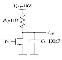
(a) Write an expression for  $I_D$  as a function of output bias point. How much does  $I_D$  change as the output voltage varies from 9V to 1V?
