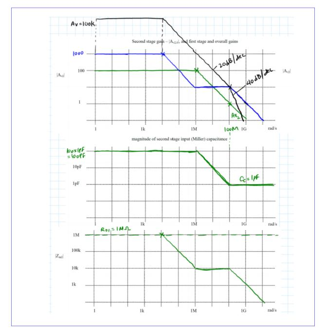
(e) What are the compensated poles of the amplifier? If  $C_c$  were 0pF, where would the poles of the amplifier be?
