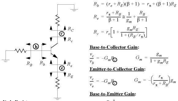
$$R_b = (r_e + R_E)(\beta + 1) = r_{\pi} + (\beta + 1)R_E$$
