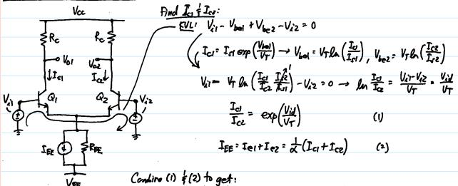
$$I_{CI} = \frac{\alpha I_{EE}}{1 + \exp(-\frac{V_{cl}}{V_T})}, \quad I_{CI} = \frac{\alpha I_{EE}}{1 + \exp(\frac{V_{cl}}{V_T})}$$
