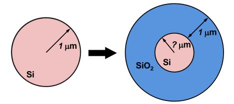
Pure silicon contains  $5 \times 10^{22}$  Si atoms per cm<sup>3</sup> and silicon oxide contains  $2.3 \times 10^{22}$  SiO<sub>2</sub> molecules per cm<sup>3</sup>. After the 1-µm-thick oxide sheath is grown, what is the radius of the silicon rod remaining in the middle? Assume that cylindrical symmetry is maintained during the oxidation.
