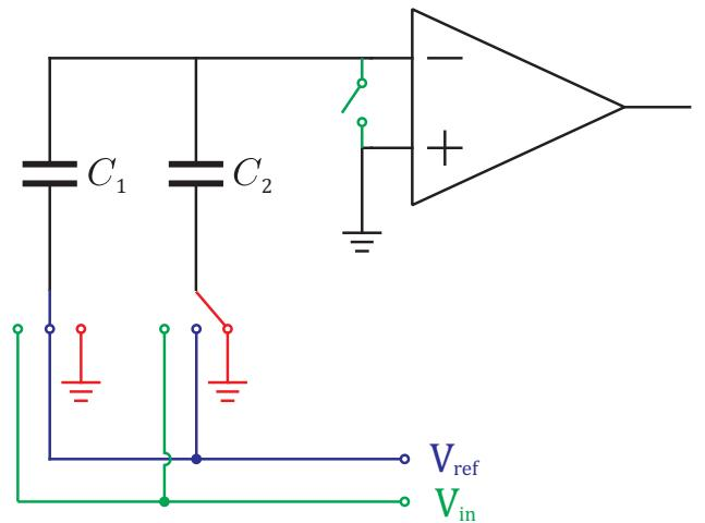
What is the comparator effectively asking? In other words, what does comparing  $V_x$  to ground imply about  $V_{in}$ , the analog signal that we care about? How does this relate to the binary search we explained before?
