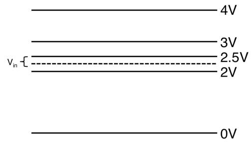
What does this binary string "1001" mean? It means  $V_{in}$  is somewhere in the range [2.25, 2.5], and the rest is up to the computer to interpret. In other words,  $1001 = 1 \times \frac{V_{ref}}{2} + 0 \times \frac{V_{ref}}{4} + 0 \times \frac{V_{ref}}{8} + 1 \times \frac{V_{ref}}{16}$ . This can also be written as (assuming BinaryRep is 1-indexed):
