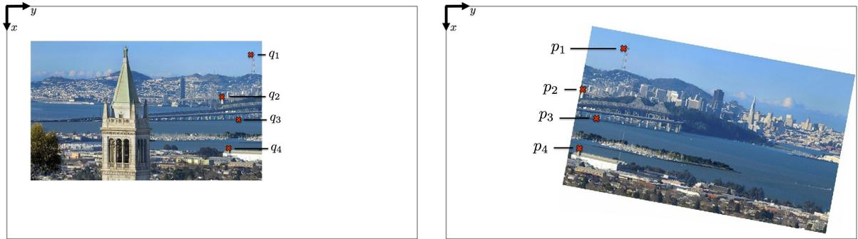
Figure 1: Two images to be stitched together with pairs of matching points labeled.
