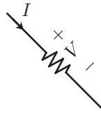
Figure 2: Current flow into a resistor results in a voltage drop proportional to the current.
