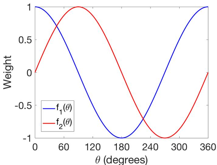
Figure 2: Weights for recorded audio signals for each of the two microphones, as a function of audio source angle  $\theta$ . Microphone 1 is blue and microphone 2 is red. Note that a weight can be negative as well as positive.
