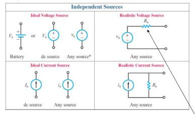
The resistance represents the fact that realistic sources "droop" when the load is increased (for example, car headlights often dim as you crank the engine to start 17
