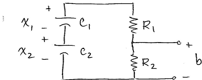
Suppose  $C_1, C_2, R_1, R_2$  are given, and  $b$  is a desired output voltage.
