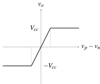
So ideally, the gain is  $A = \infty$ , input resistance  $R_i = \infty \Omega$ , output resistance  $R_o = 0 \Omega$ . A high input resistance is so we can put in the full input voltage  $v_p - v_n$ . Zero output resistance is so we get the full output voltage  $v_o$ . But why should the gain be high and why can the supply voltage be anything specified by the user?
