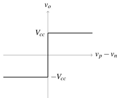
So if  $v_p > v_n$ ,  $v_o = V_{cc}$  and if  $v_p < v_n$ ,  $v_o = -V_{cc}$ . This means we can use op amps to compare the input voltage to a reference (usually ground).
