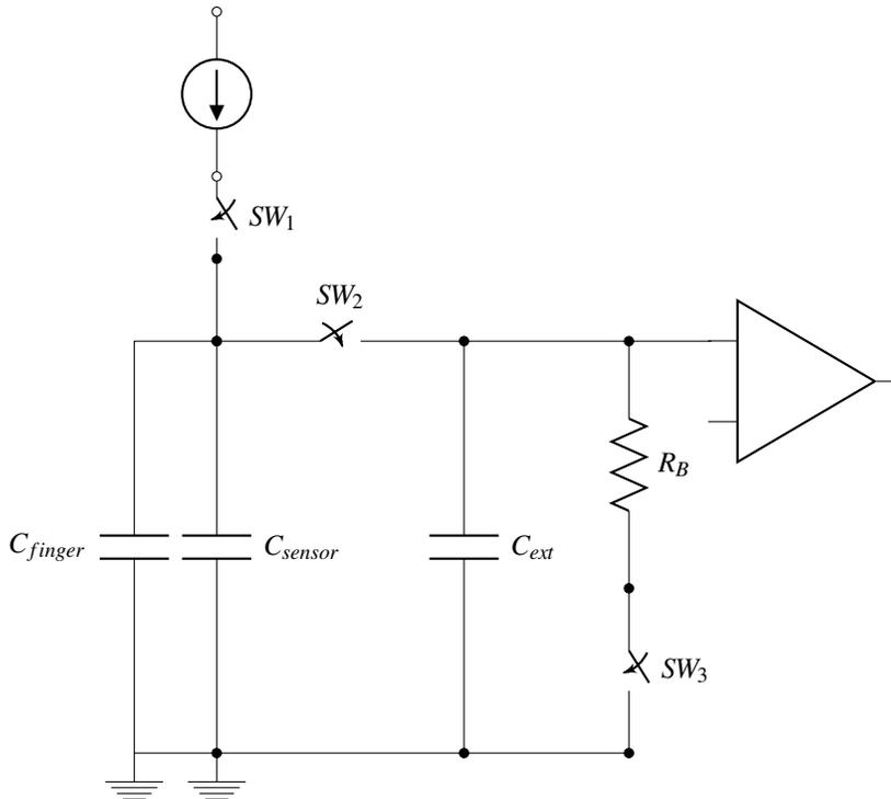
Our finger is a capacitor in parallel with  $C_{sensor}$ . This draws current away from  $C_{sensor}$ , so the change in voltage based off the first formula is lowered. This is fed to our op amp and compared to some reference voltage.
