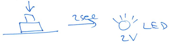
step 1: Build a ckt that after a button is pressed measures 2s and will then apply 2V across the LED.
