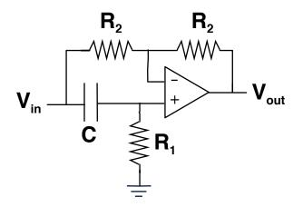
(a) Find the frequency response  $H(\omega)$  of the circuit, and sketch a Bode plot  $(20\log_{10}|H(\omega)|)$  and  $\angle H(\omega)$  versus  $\omega$ , plotted on a logarithmic scale).
