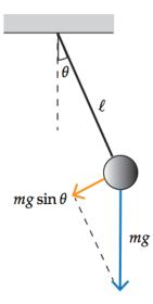
Figure 1: Pendulum Free-body Diagram
