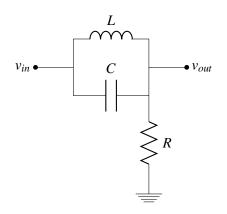
For the RLC filter above, with component values  $R = 1 \text{ k}\Omega$ , C = 1 nF, and  $L = 1 \mu\text{H}$ ,
