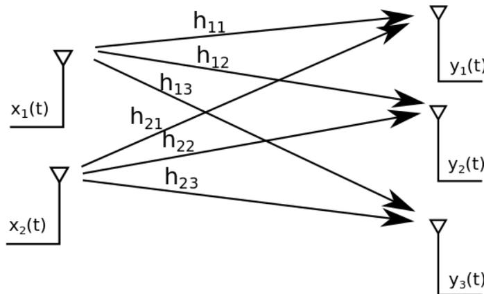
We have 2 transmit antennas and 3 receive antennas, each receive antenna gets some signal from each of the transmit antennas. We can model the input output relation of the system as follows:
