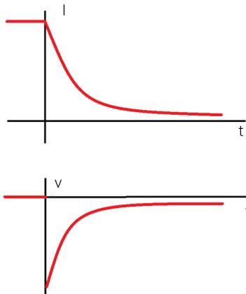
The jump we see in the voltage response is caused by the sharp discontinuity of the current.
