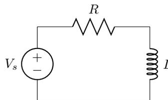
Observe the simple  $RL$  circuit above. If we replace the voltage source of an  $RL$  circuit by a short after a long period of time, what happens? Remember that after a long period of time the inductor behaves like a short.
