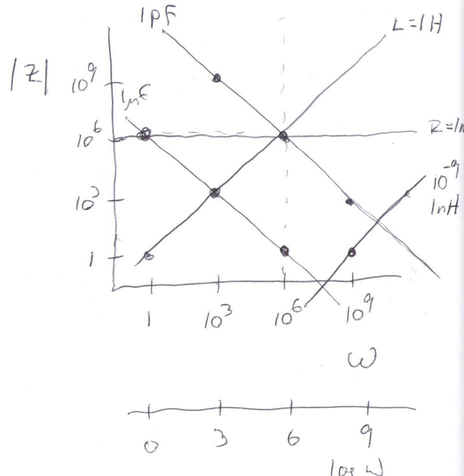
$$|Z_C| = \frac{1}{\omega C} \quad |Z_L| = \omega L$$
