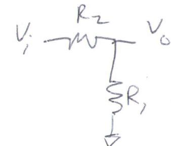
$$V_o = \left( \frac{R_2}{R_1 + R_2} \right) V_{in}$$
