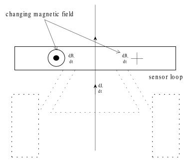
The first design has a long, rectangular loop of wire which rests on the ground in front of the car. When the car is centered around the line (as shown above), the amount of flux going through the loop sums to zero and the sensor sees a value of zero. If, as shown in the picture below, the car is slightly to the left of the wire, there will be more magnetic flux on one side than
