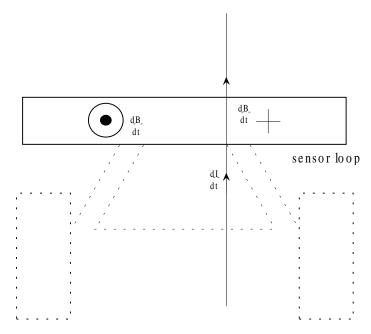
the other. Unfortunately, the track can be slanted with respect to the car such that the flux is equal on both sides. This shows that even more than one sensor is needed for detecting angle. In addition, the car will be unable to tell which way to turn even with a second, similar sensor
