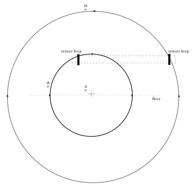
Notice that not only is the field reduced because of distance, but the percentage of the field is reduced when far from the wire because a smaller amount of the field is perpendicular to the loops.
