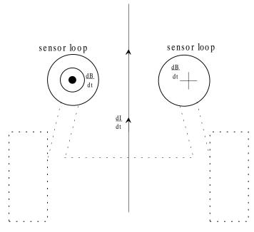
tell which side of the wire your car is on; the sensor with the largest magnetic flux will usually be
