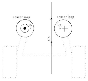
will be canceling with the flux going down, through the loop. This will cause the total magnetic flux to drop quickly as the loop passes over the wire. Of course, once the sensor has passed over
