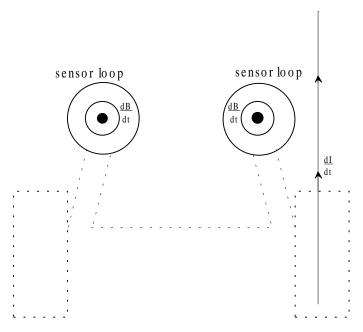
the loop, it will be possible to determine that the car is no longer in the middle of the track because the signals will no longer be out of phase as shown in the picture above. With only a pair of these sensors, the angle of the car can not be detected, so it is probably best if two additional sensors are added as shown on the next page.
