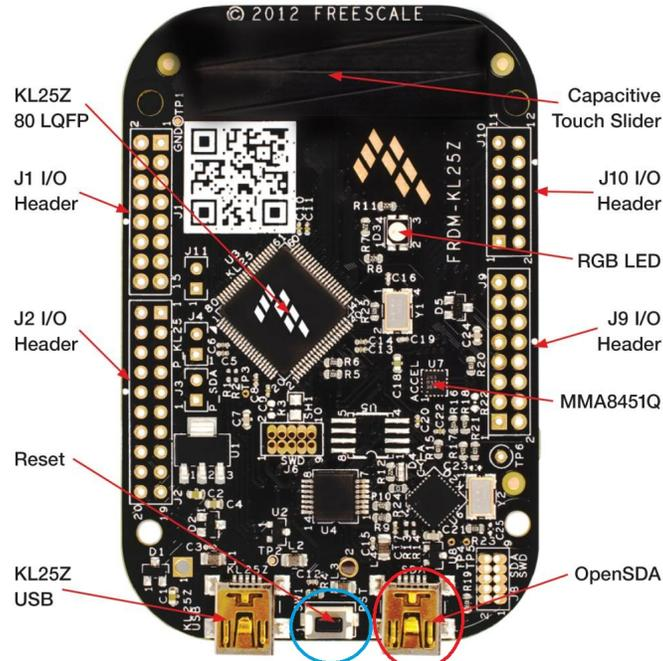
Figure 1: The Reset button circled in blue, and the OpenSDA mini USB port circled in red. The FRDM-KL25Z cannot be programmed through the other mini USB port, but it can be powered through it.
