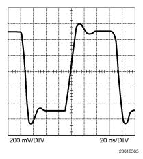
FIGURE 4. Converter Step Response (1VPP, 20 ns/DIV)
