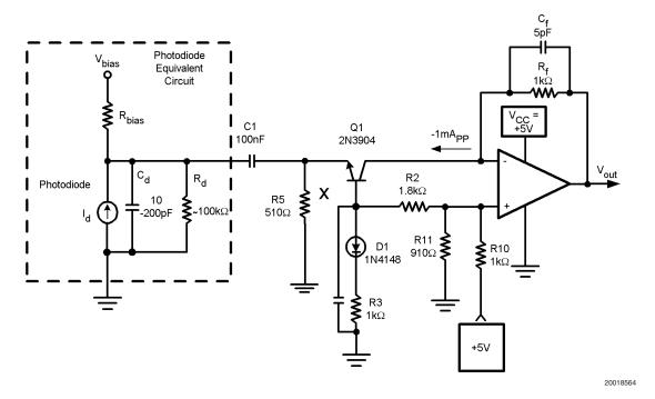
FIGURE 3. Single Supply Photodiode I-V Converter
