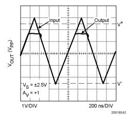
FIGURE 1. Input and Output Shown with CMVR
