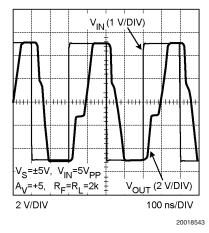
FIGURE 2. Overload Recovery Waveform
