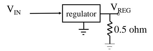
Linear Regulator  $V_{IN} > V_{REG}$
