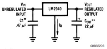
\*Required if regulator is located far from power supply filter.
