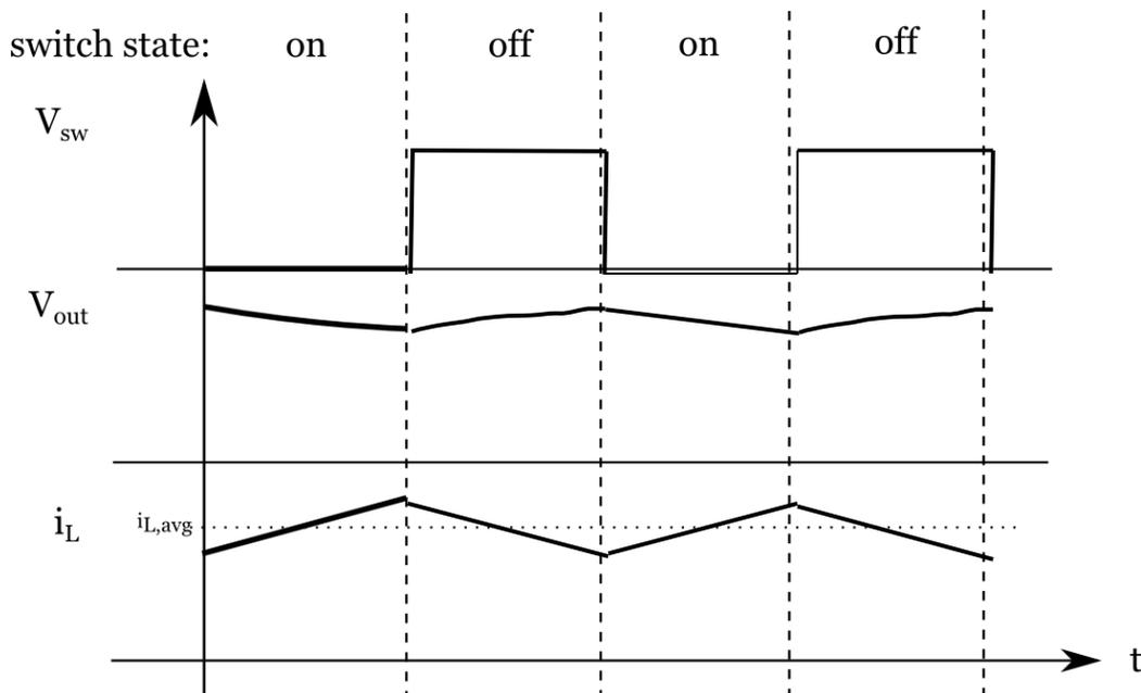
For simplicity, assume  $i_L$  goes from  $i_{\max}$  to  $i_{\min}$  in a linear fashion in time  $T_{\text{off}}$ , with a change of  $\Delta i = i_{\min} - i_{\max} (<0)$ . Also assume  $V_{\text{out}}$  is approximately constant. During  $T_{\text{off}}$  the instantaneous power delivered to the capacitor and load from the inductor in series with  $V_{\text{in}}$  is  $p(t) = i_L(t) (-V_L(t) + V_{\text{in}})$ .
