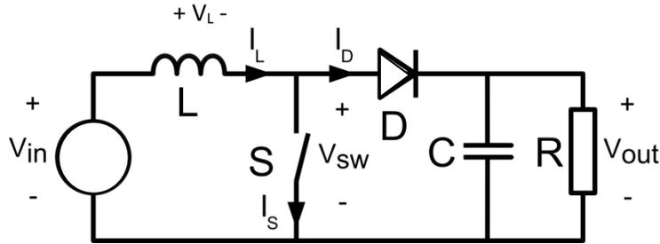
1. Fill in the plots for two periods of the boost converter's operation.
