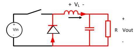
Output voltage is less than input voltage
