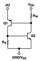
Figure 3. Rearrangement of the way we view the parasitic bipolars of Figure 2 shows an SCR structure.
