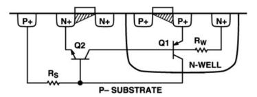
Figure 2. Cross-section of PMOS and NMOS devices, showing parasitic transistors Q1 and O2.
