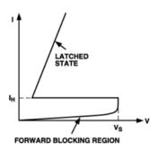
b) Current- voltage characteristic of an SCR.
