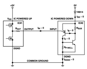
Figure 4. Addition of a diode in series with V<sub>DD</sub> prevents SCR triggering.
