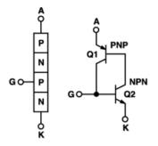
a) Transistor equivalent of an SCR.
