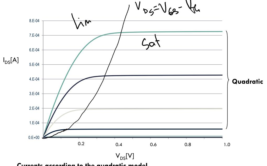
Currents according to the quadratic model Correct for long channel devices (L  $\sim \mu m$ )
