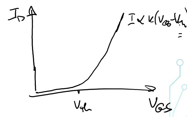
$\int_{-\infty}^{\infty} K(V_{GS} - V_{THZ}) \text{ Model } (\alpha = 1)$
