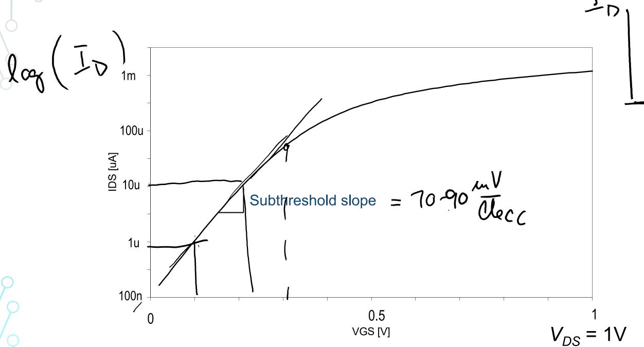
Leakage current is exponential with  $V_{GS}$
