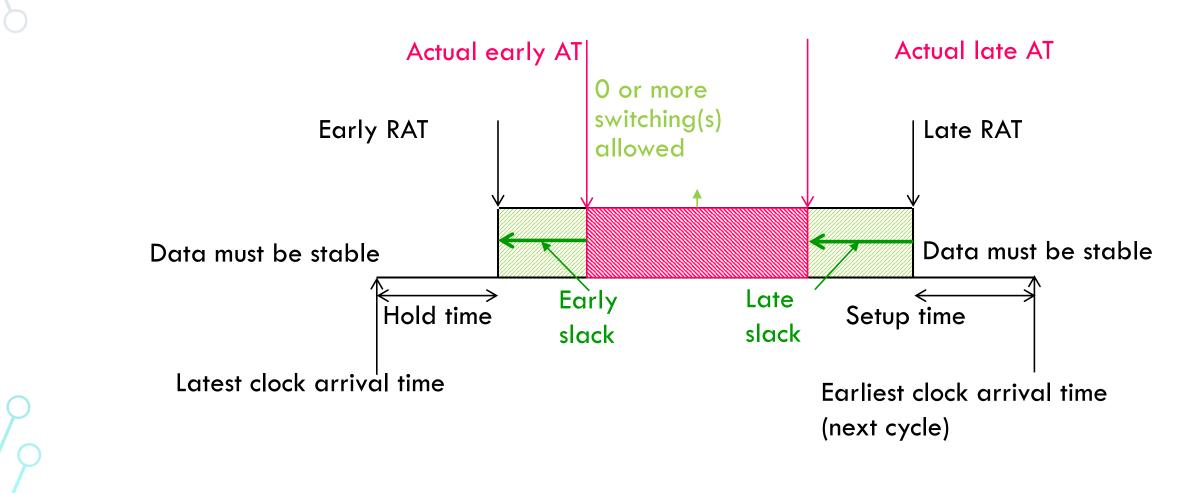
EECS241B L09 FLIP-FLOP TIMING
