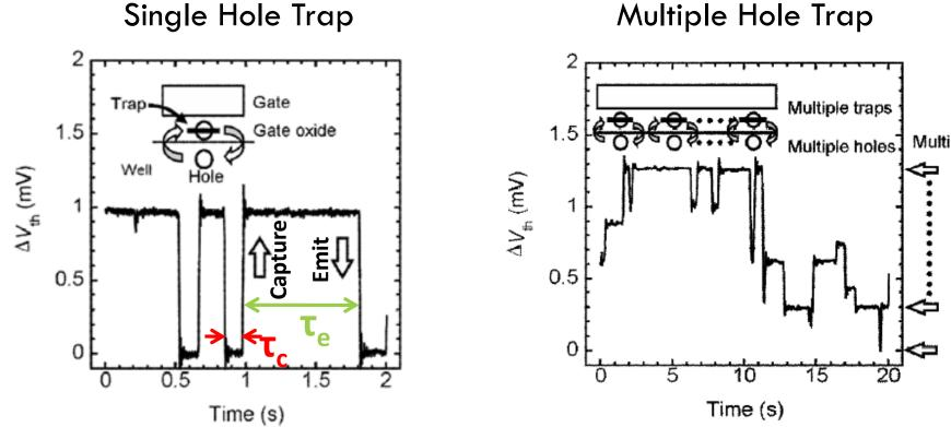
• Trapping of a carrier in oxide traps modulates  $V_{th}$  or  $I_{ds}$
