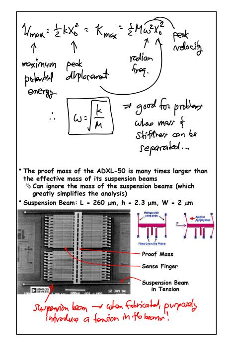
**Tethers** with fixed ends. Applied Acceleration **Fixed Capacitor Plates** mac of structure (shuffle) >> mous of springer ignore the mass of the springs stiffing of the springs << stiffness of shuttle is ignore the officers of the shall Fat 6 ADXLJO: M= 162 ng ~ 50% of this is in the fingers! Suspenden: four fenning become Gyldd B.C. Fixed B.C. Kc F/4 Bending compliance  $k_{h}^{-1}$ F/4 ĸ Stretching compliance  $k_{st}^{-1}$
