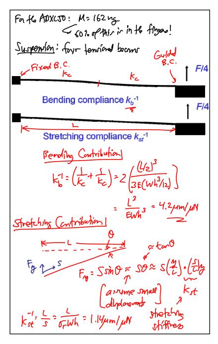
To got to total spring constant add to bending shifties to be spetching: k=4(kb+kg+)=4(0.24+0.88)=4.5 MN/um Now, got the resonance frog .: f: 211/k = 1 (4.5 N/m) = 26.5k/2 ADXL-50 Data Sheet: fo = 24 kHz & difference? capacitive transducen 1 shift freg. introduces a regative SHAffres, ke andrial stiffres.
