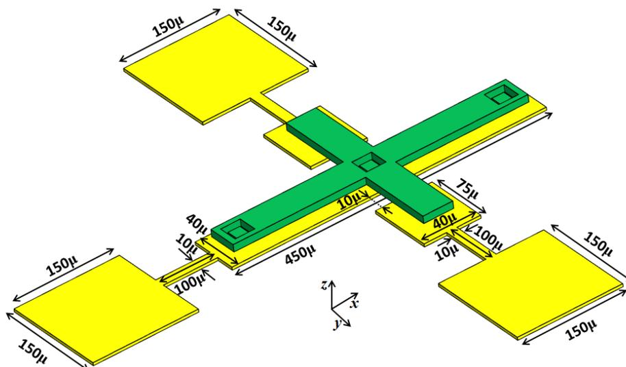
Fig. PS5.1-2: Wide-view schematic with electrode contact dimensions
