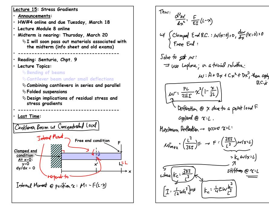
Ex: L= 10 yum, W. Zum, h= Zum polysilica - E: 150 GPg  $t_c = \frac{1}{4} (150G) (2\mu) \left(\frac{2\mu}{100\mu}\right)^2 = 0.6 N/m$ Maximum Stracs in a Bost Comilone From bofne, the redius of curvature is given by = = is movimized (i.e., R is minimized) when X:0 (x:0]= I dw FL R dw FL 1:0 Strain is maximized: 1) At the top surface - fonile (2) At the bottom surface -+ compressive Emax: 2 = h 1: (h FL = Emax) [I: 12Wh3] = Emox = K FC (12) = (6L EWh2F = Emox
