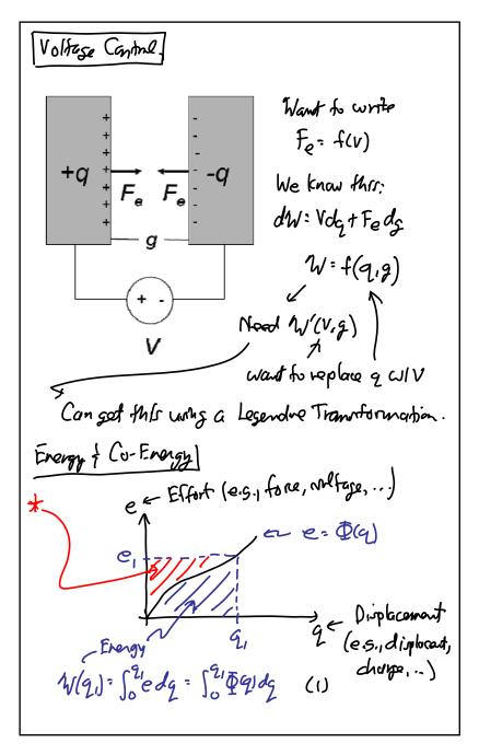
Co-Enorgy: \*  $W'(e_1) = \int_{0}^{e_1} q de : \int_{0}^{e_1} \Phi^{-1}(e) de$  (2) For a libear system, (1) { (2) will be equal. Can define cu-energy as: W(e) = eq - W(q) (from the plot) (O May Co-Energy Formulation for Voltoge Control  $\mathcal{W}(v,g): Vq - \mathcal{W}(q,g)$ +q + F. F. -q Differentially, this becomes. Workins V dW (Vis)= (qdv + Vdg)- dW(qis) Co-Frongy Expression [dW(q,s): Fedgt Vdq] d'w'(Vig): qdV-Fedg
