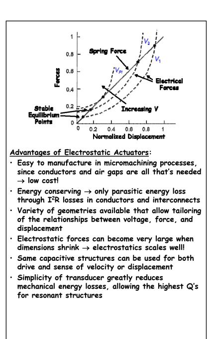
Disadvantages of Electrostatic Actuators: • Nonlinear voltage-to-force transfer function • Relatively weak compared with other transducers (e.g., piezoelectric), but things get better as dimensions scale Variable Nononclature VanNA VA Composit Va 7+  $V_a = N_A = V_A + N_a$ Ns N¢
