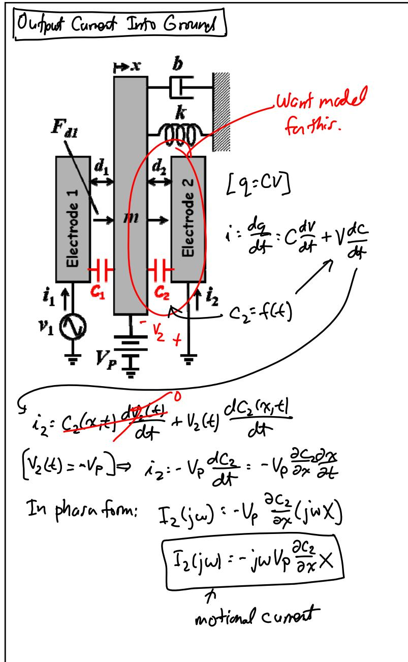
$$I_2(j\omega) = -j\omega V_p \frac{\partial C_2}{\partial x} X = -V_p \frac{\partial C_2}{\partial x} \dot{x}$$
