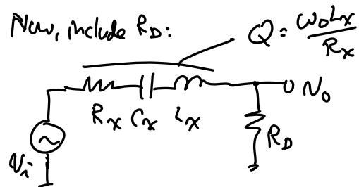
$$\frac{V_o(s)}{V_i(s)} : \frac{R_D}{R_D + R_x + \frac{1}{sC_x} + sL_x} = \dots \text{math} \dots$$
