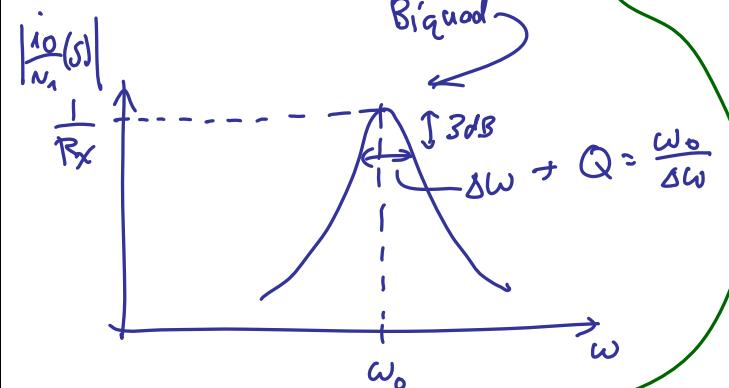
Significance: Can just solve the clst. @ resonance, then multiply by a proper  $H(s)$ !
