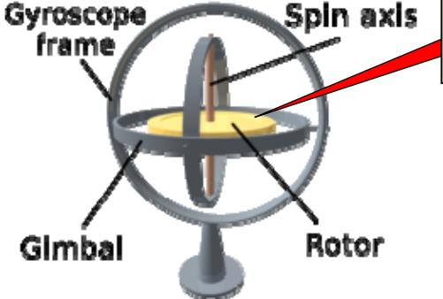
Rotor will preserve its angular momentum (i.e., will maintain its axis of spin) despite rotation of its gimbaled chassis
