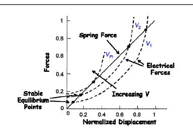
Advantages of Electrostatic Actuators:
