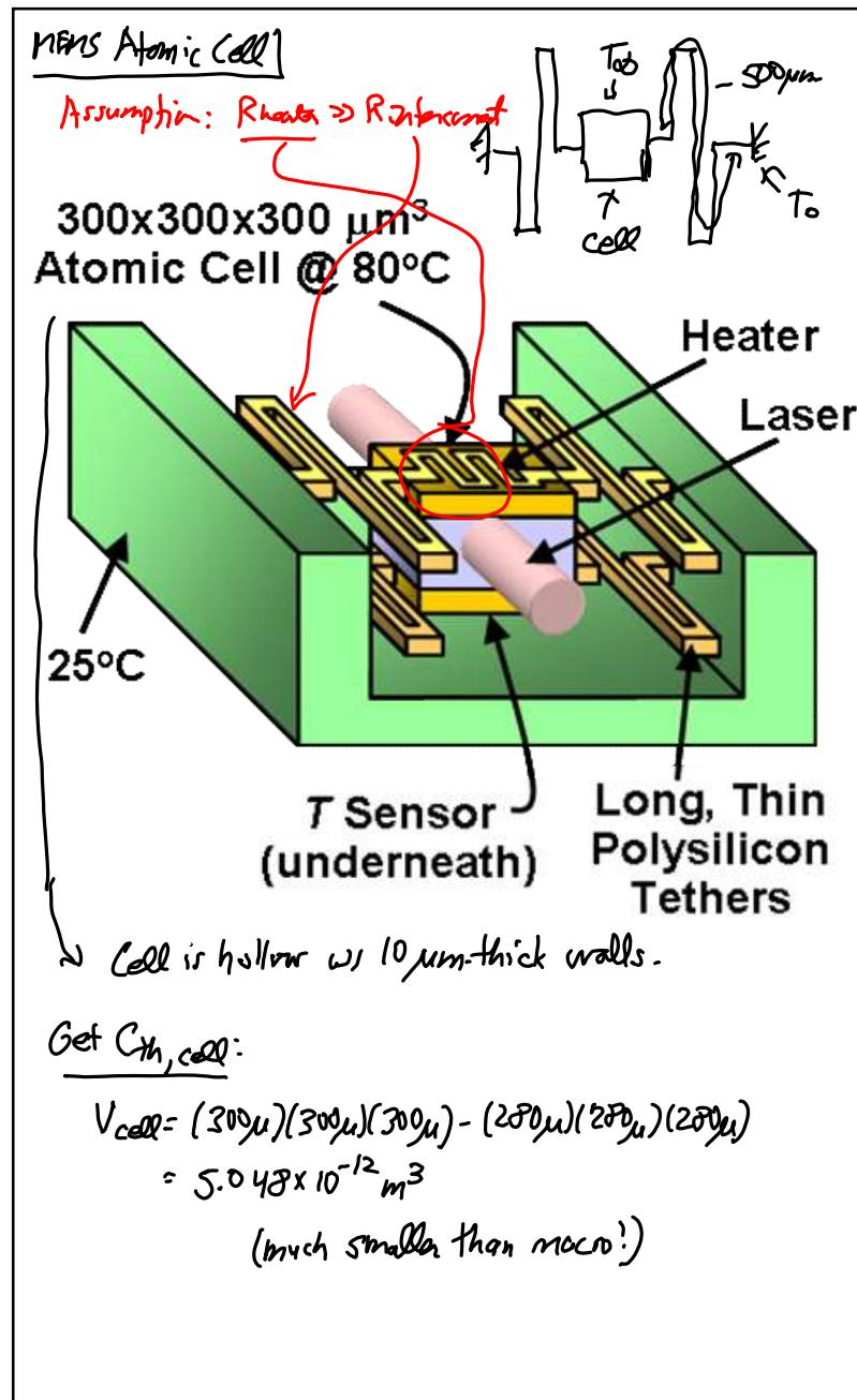
$$C_{th,cell} = \rho_{\text{glass}} V_{\text{cell}} C_{p,\text{glass}}$$
