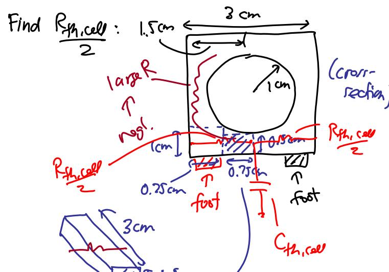
$$\frac{R_{th,cell}}{2} = \frac{\frac{3}{4}}{k(3)(\frac{1}{2})} + \frac{\frac{3}{4}}{k(3)(1)} = \frac{1}{k} \left( \frac{1}{8} + \frac{1}{4} \right) = \frac{3.1}{8k}$$
