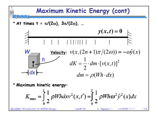
• Equate the maximum potential and maximum kinetic energies:  $K_{max} = \int_{0}^{L} \frac{1}{2} \rho W h \omega^{2} \hat{y}^{2}(x) dx = W_{max}$ • Rearranging yields for resonance frequency: w = resonance frequency  $w_{max} = maximum potential energy$   $\rho = density of the structural material$  W = beam width h = beam widt
