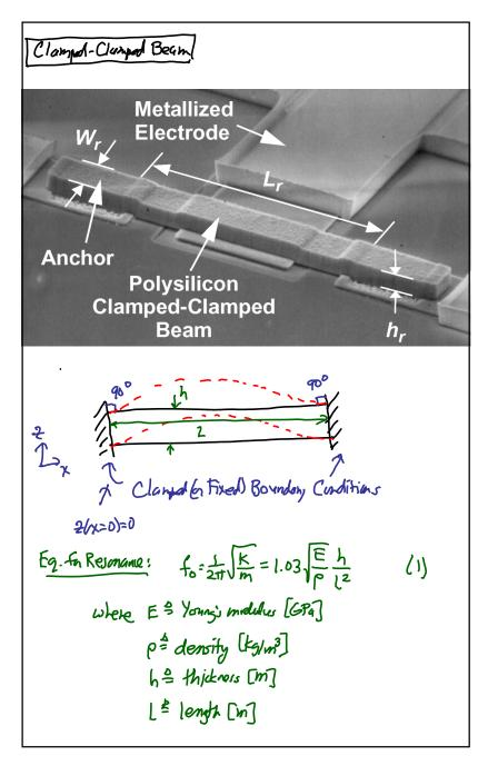
Example. 1=40 m, h= Zum polysi: E=150 GPa, p: 2300 kg/m3 :. fo: (1.03) \[ 1526 \frac{2\psi}{49\psi\psi} \Rightarrow \frac{10.4MH2}{2300} \] VE & acoustic volveity 8076 mis Lnew & S. Lold Scalingi 1) Scale all dimonsions equally by a factor S: fo~ 5 ~ t (but... problems...) Example. L=4 µm - fo= (1.03)(8076) (4n)= fo= 1.046Hz
