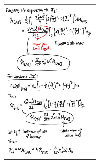
and Rhax: Xowo (= hs + = Me + = Ms) for the total nechanical de both truces Call beams Wmax - max. potential enorgy - equel to the work done to achieve maximum deflection  $W_{max} = \frac{1}{5}k_{x}\chi_{p}^{2}$ Then, using Rayleigh - Ritz:  $W_0 = \left[\frac{k_c}{Meg}\right]^{\frac{1}{2}}$ where  $M_{eq} = M_{s} + \frac{1}{4}M_{t} + \frac{12}{35}M_{b}$ (Resonance Freq. of a Folded-Beam) Suspended Shuttle
