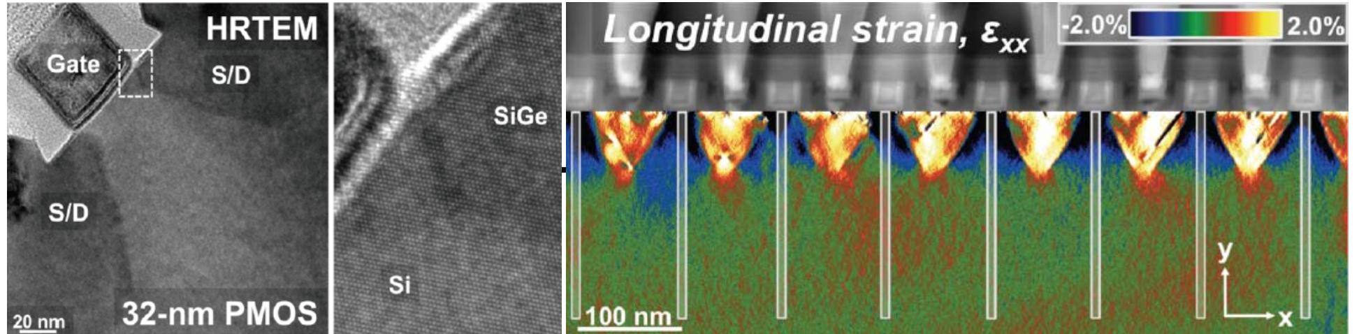
Strain mapping from a 32nm node PMOS. Courtesy of B. Özsdöl (LBNL)
