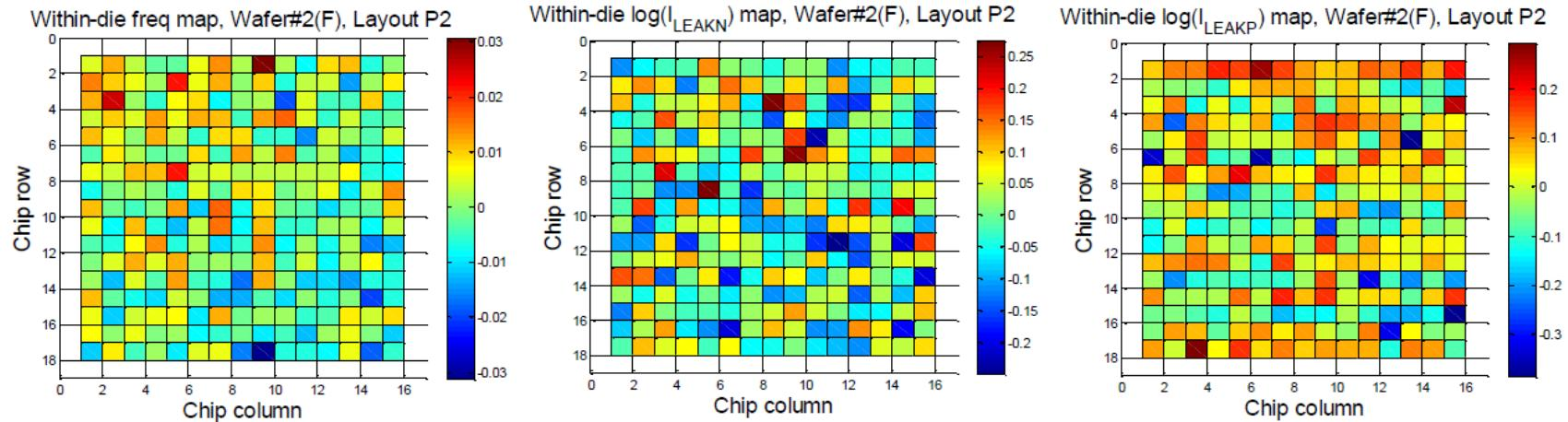
45nm Bulk CMOS Within-Die Variations. Courtesy of C. Spanos (UC Berkeley)
