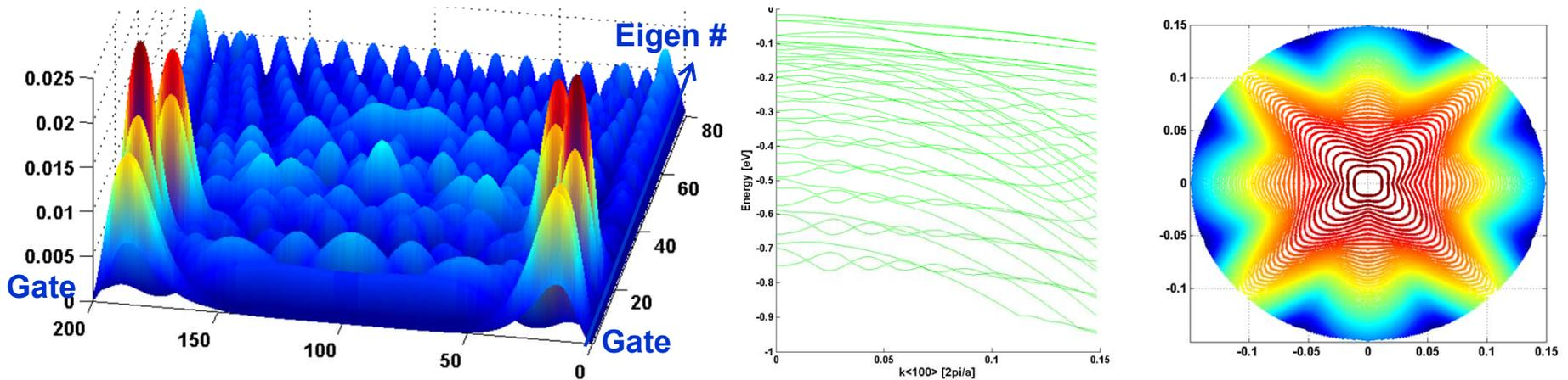
Hole's Wavefunctions,  $E$ - $k$  and Equi-Energy Contours from a P-FinFET
