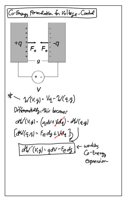
Find co-energy in terms of voltage, V: W'= 5 9(9, V') dV'= 5 (EA) V' dV' =  $\frac{1}{2} \left( \frac{\epsilon A}{4} \right) V^2 = \frac{1}{2} C V^2 \sqrt{\text{(as expected)}}$ Electrosfetic (a Voltage - Carinllad) Force: Fe: - 2W (V,g) (V=const = - \frac{1}{2} \left( \frac{\xi A}{9^2} \right) V^2 = \frac{1}{2} \frac{\xi V^2}{9} Fe \right]
