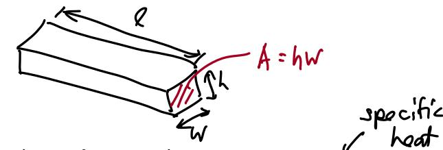
$\Rightarrow \text{thermal capacitance: } C_{th} = \rho V C_p$
