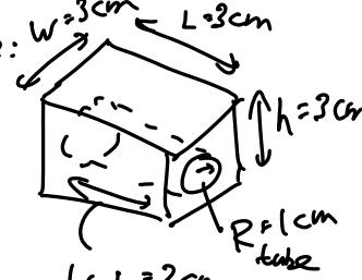
$$C_{th,cell} = \rho_{glass} V_{cell} C_{p,glass}$$
