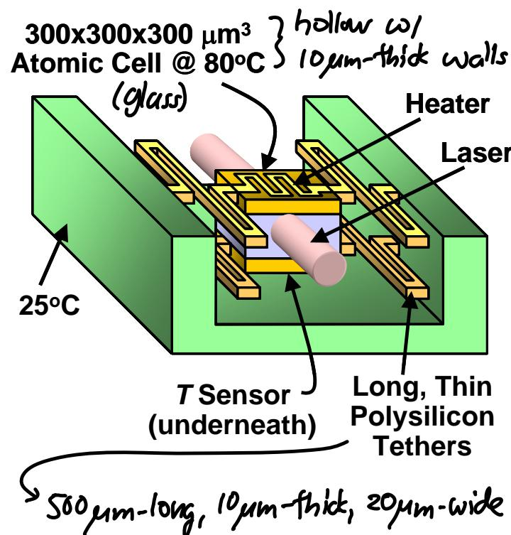
$$V_{cell} = (300 \mu\text{m})(300 \mu\text{m})(300 \mu\text{m}) - (280 \mu\text{m})(280 \mu\text{m})(280 \mu\text{m}) \\ = 5.048 \times 10^{-12} \text{ m}^3$$
