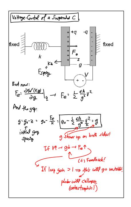
Change: (for a stall gap) 9: 2W'(V,g) / = CV Stability Analysis => deference under what conditions voltage-control will cause collapse of the plater: Find: Fe-Fipping:  $\frac{\epsilon Av^2}{2g^2}$  -  $k(g_0 - g)$ What happear whom g changes by incoment of?
