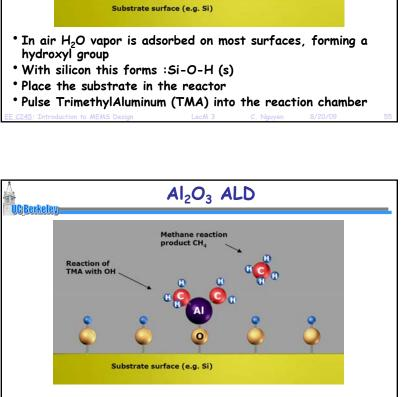
TrimethylAluminum (TMA) reacts with the adsorbed hydroxyl groups, producing methane as the reaction product
