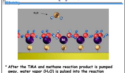
away, water vapor  $(H_2O)$  is pulsed into the reaction chamber.
